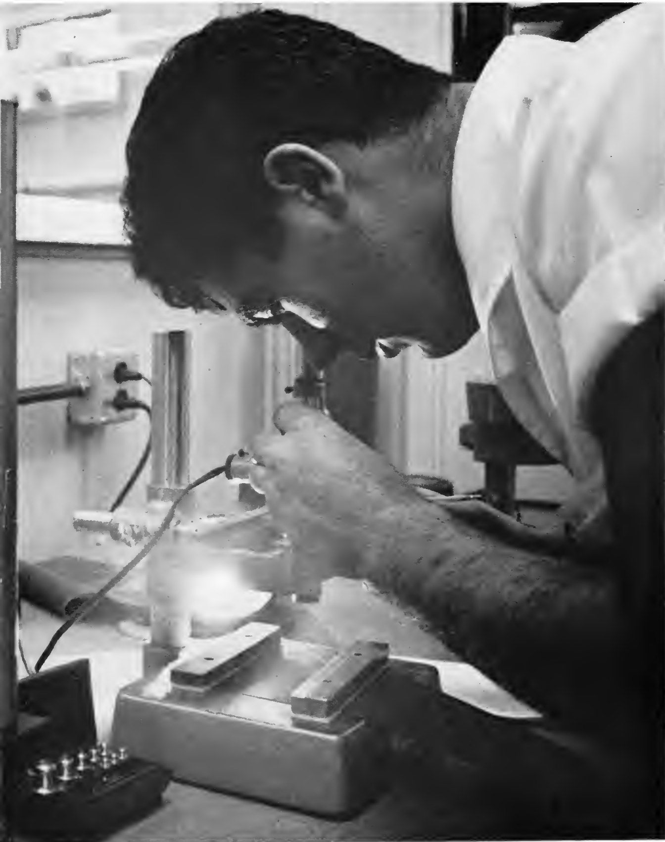
AUDIO DEVICES technician at the company's plant in Stamford, Connecticut checks sample of Audiotape under microscope for possible width variation. This is just one phase of quality checking during production at Audio Devices. All Audiotapes—including Audio's extra precision tapes for instrumentation and computer use — are also checked for uniformity, sensitivity, frequency response and distortion. EP Audiotapes are 100% certified against signal drop-out.
